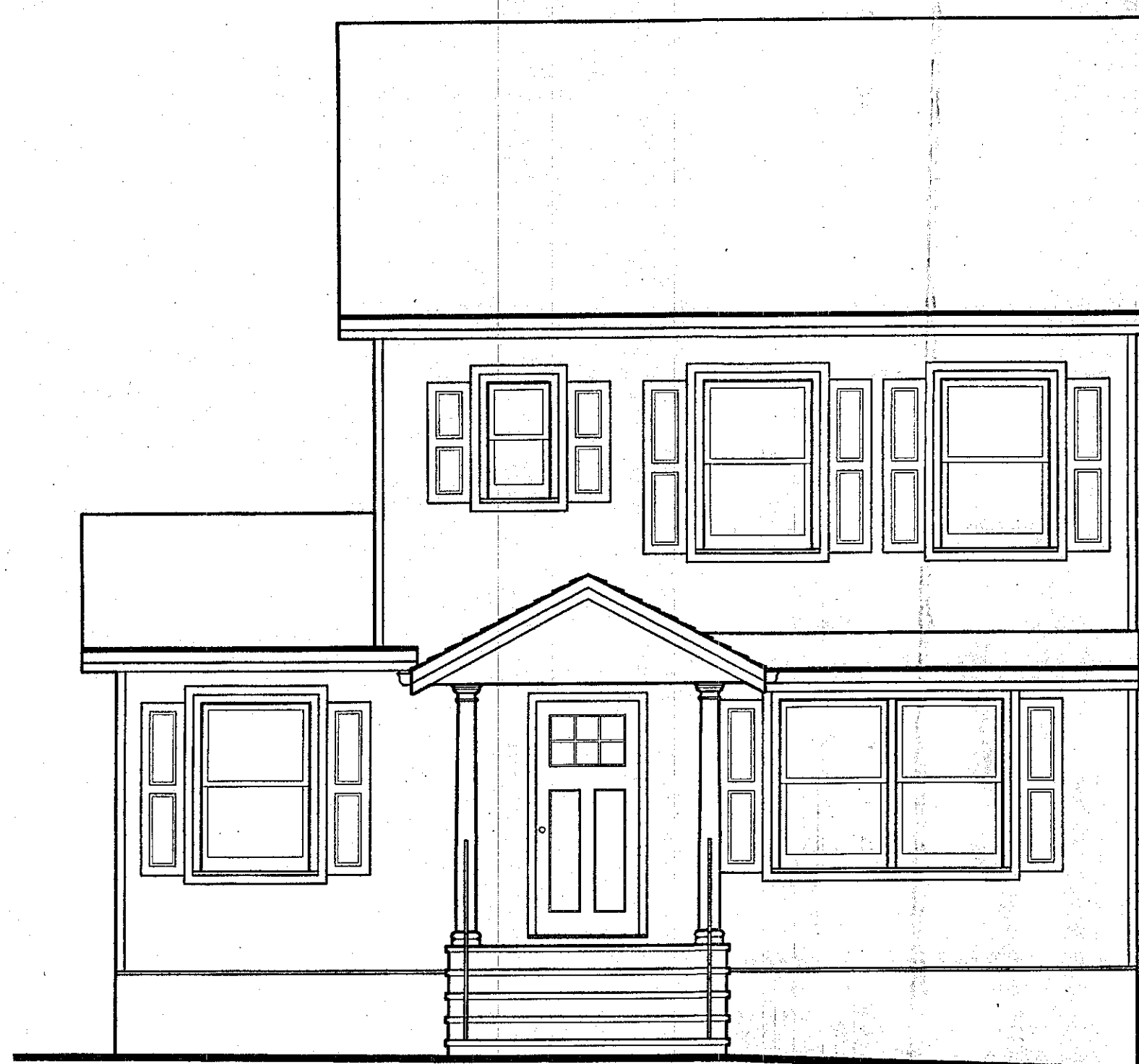
(A) EAST ELEVATION - EXISTING SCALE: 1/4" = 1'-0"
